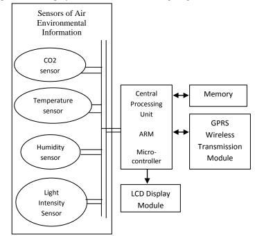
Figure : Hardware infrastructure diagram of geological CO2 leakage monitor
